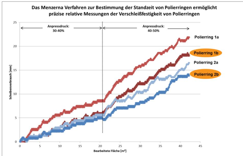
Fig. 2: Wheel wear as a function of the polished area at two different contact pressures.
