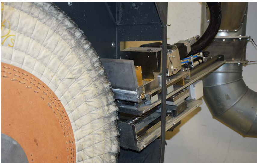
Figure 3: MELT Dosing head integration into an existing polishing system
