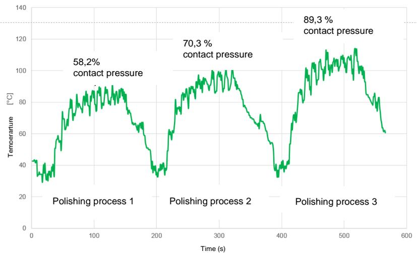
Figure 1 Temperature development in the robot cell during three polishing cycles with 10 passes each and different contact pressures
