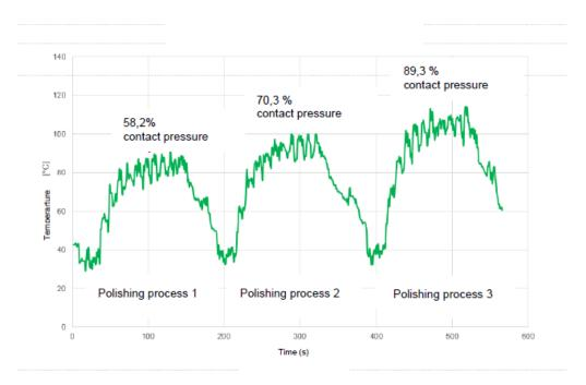
Figure 1 Temperature development in the robot cell during three polishing cycles with 10 passes each and different contact pressures
