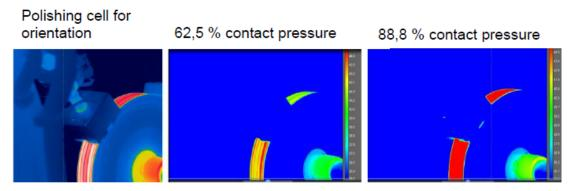
Figure 2 Temperature development on the polishing wheel during the polishing process with various contact pressures
